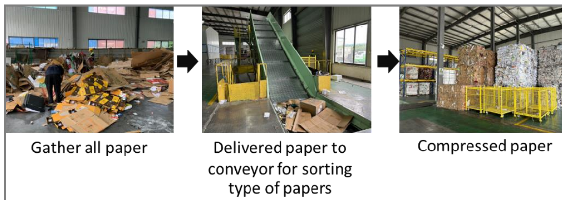
Figure7- 2-12 Paper Type Recycling Waste Management Process at Baiyangwan Sorting Center
