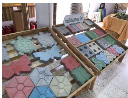
Figure 7-2-3 Bricks made from Plastic Scrap Ban Eua Artorn Community Center Rayong (Wang Wa)
